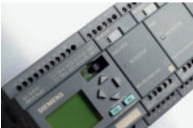
LOGO! in assemblies with the function modules
